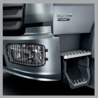
Geared to operational needs. The moving entrance step on the Atego all-wheel-drive variants illustrates how the new Atego is geared to specific operational needs. And details such as the optionally available headlamp protection grilles prevent damage while at the same time enabling swift and simple cleaning of the headlamps
