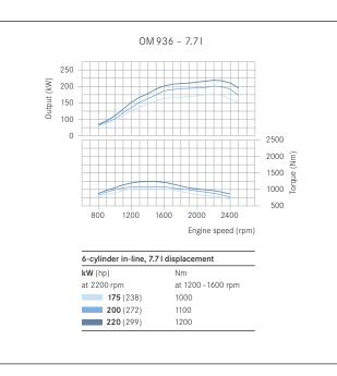
More power, more torque. With an output of up to 220 kW (299 hp) and up to 1200 Nm of torque, the new 6-cylinder in-line engines provide just the power you need for your operations in the building materials industry
