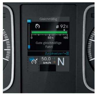
FleetBoard® EcoSupport. While the driver is at the wheel, the standard-fit FleetBoard® EcoSupport system provides him with a steady output of tips on how to further optimise his driving style in the interests of reduced fuel consumption and wear
