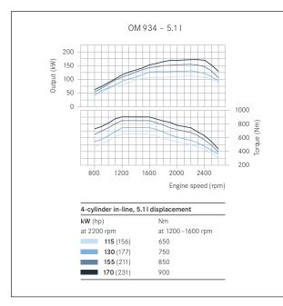
Reduced displacement, increased performance. With an output of up to 170 kW (231 hp) and maximum torque of 900 Nm, the Atego's new 4-cylinder in-line engines boast performance data which have been the reserve of 6-cylinder engines to date
