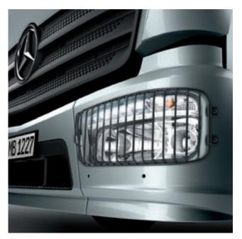
**LED technology.** Apart from highlighting the Atego's distinctive design, the optionally available LED daytime running lamps also cut costs, as the LEDs are designed to last throughout the Atego's useful life. LED side marker lamps and tail lamps are optionally available
