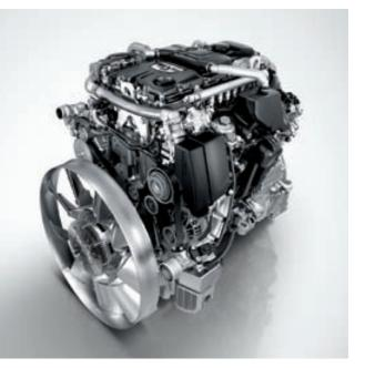
Engine portfolio. With an output of up to 170 kW (231 hp) and up to 900 Nm of torque, the new 4-cylinder in-line engines of the OM 934 series offer ample power for practically any task in the building materials industry. The new 6-cylinder in-line engines of the OM 936 series offer even more power and torque
