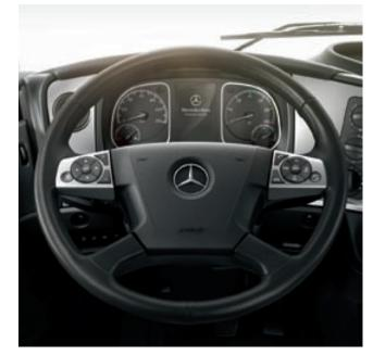
Multifunction steering wheel. The standard-fit multifunction steering wheel makes light work of various functions: apart from the radio and telephone, the cruise control can now also be operated via the steering wheel. Many other vehicle functions and diverse settings can also be controlled in the new instrument cluster
