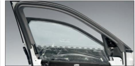
Window lift system and side windows integrated using specific process - front and rear windows almost fully lowerable
