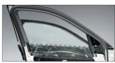
Window lift system and side windows integrated using specific process front and rear windows almost fully lowerable
