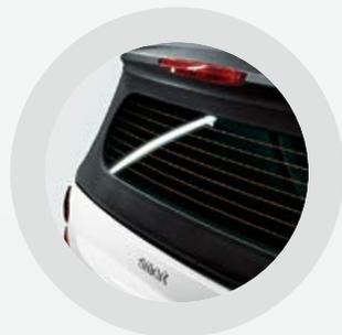
**Glass rear window:** the cabrio's rear window is made of scratch-resistant safety glass. And it's heated – for maximum safety in every weather.
