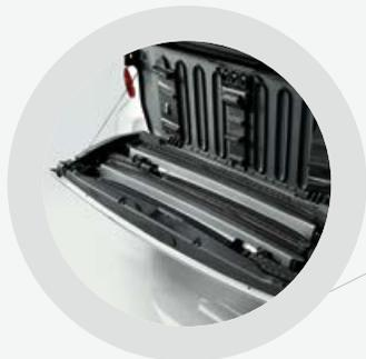
**Tailgate with storage compartment for side bars:** for maximum open-air driving pleasure you can remove the side bars and stow them away in the special compartment in the tailgate. Alternatively, an insert for the charging cable can be ordered at no extra charge.
