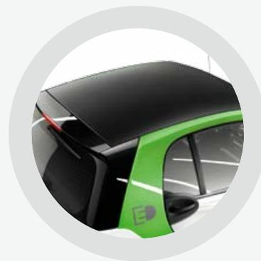
**Solid roof:** the coupé comes with a black solid roof as standard. The robust plastic has a structured surface, making it particularly hard-wearing.
