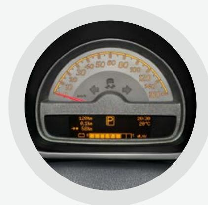
**Instrument cluster with trip computer display:** the multifunctional display has a READY indicator that shows when the vehicle is ready to go. It also comprises an ECO display for optimising the driving style, a remaining range indicator, settings for departure and charging time, settings for pre-entry climate control and service interval indicator.
