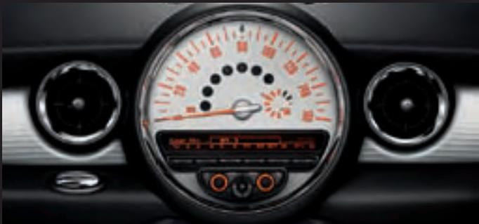
The large **speedo** in the middle of the instrument panel includes warning and indicator lights and the fuel gauge.
