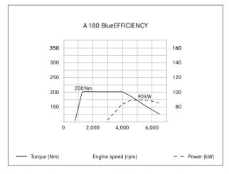
The A180 4-cylinder petrol engine benefits from direct petrol injection, variable valve timing and turbocharging
