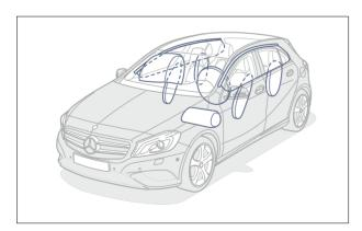
Windowbags for front and rear seat occupants, front airbags and sidebags and a driver's kneepag are all fitted as standard
