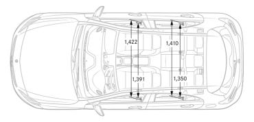
All measurements in millimetres. The dimensions shown are mean values and apply to standard-specification, unladen vehicles
