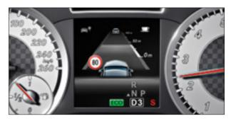
Speed Limit Assist shows the permitted maximum speed in the instrument panel and on the COMAND Online display
