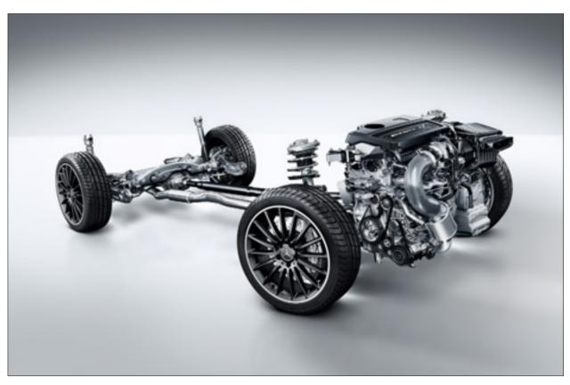
AMG-specific elasto-kinematics increase dynamism through stiffer axle bearings
