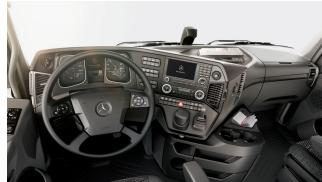
**BigSpace cockpit.** With a width of 2500 mm and a completely flat floor, the BigSpace cabin (shown here in Arocs trim) provides an impressive working atmosphere with living, working, and storage space in abundance.
