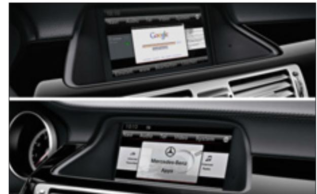
SplitView shows two screens simultaneously, allowing driver and front passenger to view different content
