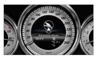
Active Park Assist displays the status of the parking manoeuvre in the instrument panel
