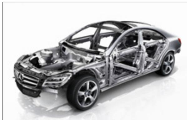
The energy-absorbing front and rear crumple zones, a highly rigid passenger compartment and internally reinforced doors provide highly effective protection in the event of an accident
