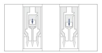
Direct Control suspension adjusts the damping automatically as you drive, ensuring high levels of comfort and agility at all times
