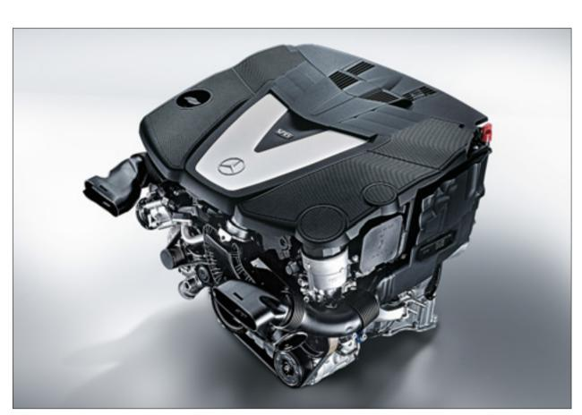
The CLS 350 CDI engine, with 265 hp (195 kW) power output
