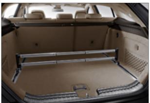
The load area with optional Easy-Pack load-securing kit (Shooting Brake only)
