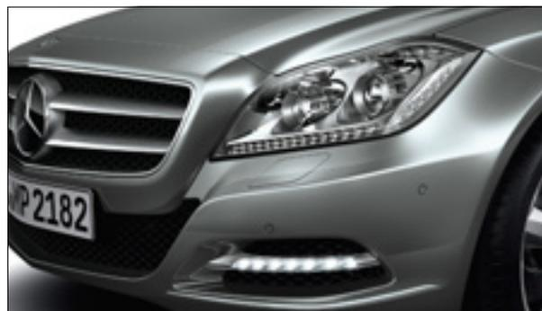
Bi-xenon headlamps with LED daytime running lights are fitted as standard
