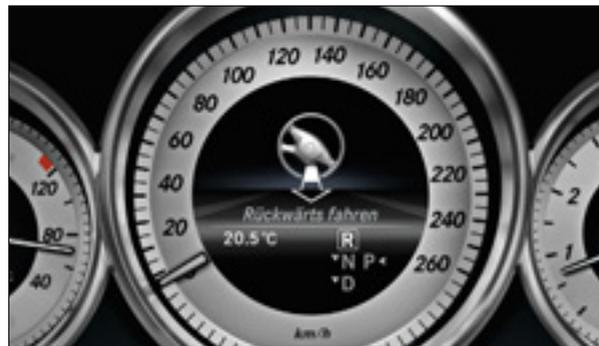
Active Park Assist displays the status of the parking manoeuvre in the instrument panel
