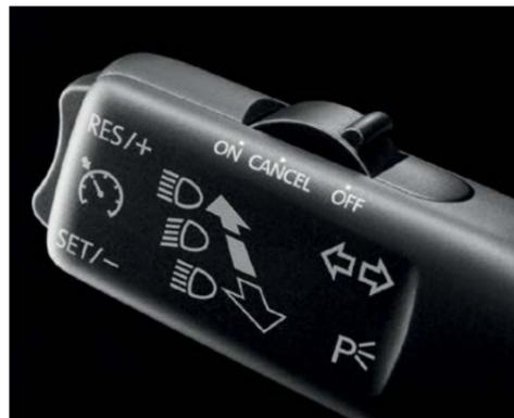
**Cruise control** can be set at speeds of over 19mph to maintain a constant speed. Once set to your desired speed, all your concentration can be focused on the road ahead creating a more relaxed drive. Optional on Beetle, Beetle Cabriolet and Design, and standard on all other models.
