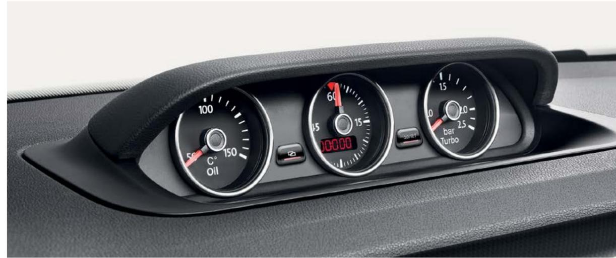
The **three dial 'Sport' instrument panel** on the dashboard is a particularly distinctive feature showing information about oil temperature and turbocharger boost, as well as the multifunction stopwatch that can measure the journey time and time stopped. Standard on Sport, Beetle Turbo Black and Turbo Silver, and optional on all Design models.
