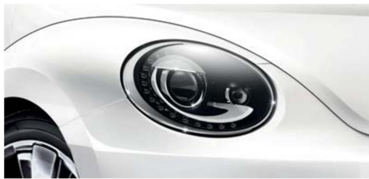
**Gas discharge (Bi-xenon dipped and main beam headlights)** including range adjustment and LED daytime running lights ensure your vehicle is visible to other road users in any weather. Optional on all models.
