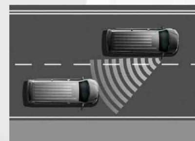
**Lane Change Assist<sup>1,2</sup>** has radar sensors to help monitor traffic. When you change lanes, the system warns you via flashing lights in the exterior mirrors if another vehicle is identified within the blind spot.
