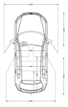
On illustrations, where arrows and figures are shown inside of the vehicle, the measurements are for interior dimensions. Where arrows and figures are shown outside of the vehicle, the measurements are for exterior dimensions.
