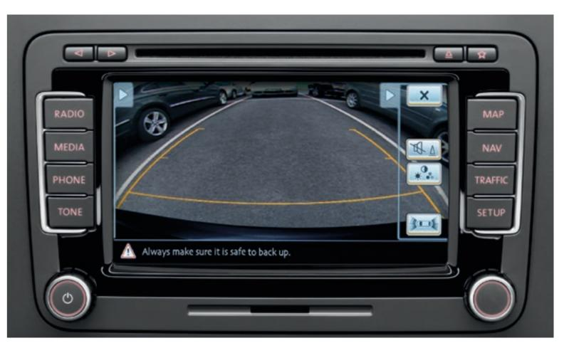
() The rear-view camera, shown here as part of the RNS 510 touch-screen DVD navigation/DAB radio system option, is located in the rear tailgate and reproduces an electronically straightened image on the audio system's display. This provides an unobscured view to the rear of the vehicle, making parking easier and safer, even when towing a trailer.
