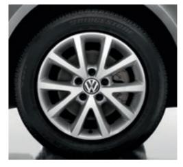
🔊 🕸 🕪 16 inch **'Perth'** alloy wheels with 205/55 R16 tyres give a touch of individuality to your Touran and are protected by anti-theft wheel bolts. BlueMotion Technology models feature 205/55 R16 low rolling resistance tyres as standard.
