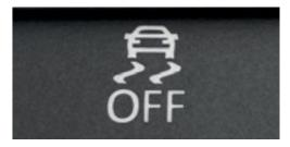
**GG** The Electronic Stability Control (ESC) utilises sensors to detect critical situations at an early stage, reacting within milliseconds by controlling the speed of individual wheels, helping to bring the vehicle under control.
