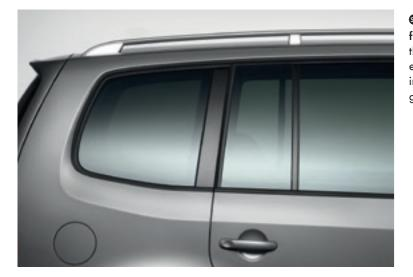
**G** The heat insulated rear tinted glass from the B pillar backwards reduces the glare of sunlight by up to 65%, ensuring a pleasant interior temperature in the passenger compartment and giving occupants additional privacy.
