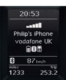
(5) **G** Bluetooth telephone connection for HFP (Hands Free Profile) enabled telephones allows you to use your phone safely whilst driving. The phone book and call information is displayed on the audio system's display and on the multifunction computer.
