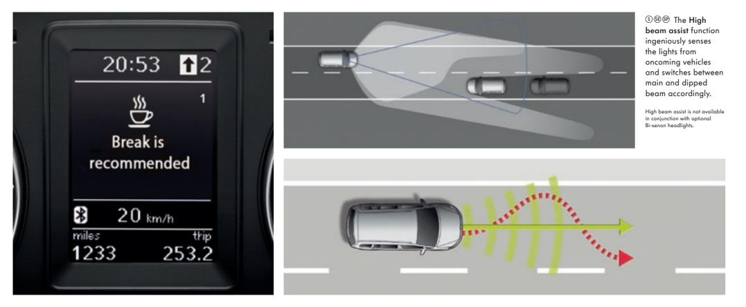
The Driver Alert system detects when the driver is becoming tired and recommends taking a break. This is achieved by monitoring driving behaviour closely, noting any erratic steering wheel movement and alerting the driver via visual and audible warnings.
