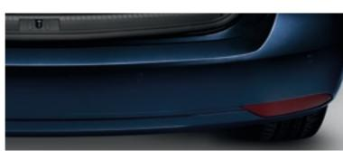
(5) (5) (5) Rear parking sensors, are ultrasonic, audible with audio volume reduction when activated and optical parking display via vehicle's audio system.
