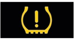
**G G G** In the event of a change in air pressure, the tyre pressure loss indicator symbol appears in the multifunction display, advising the driver to rectify the situation.
