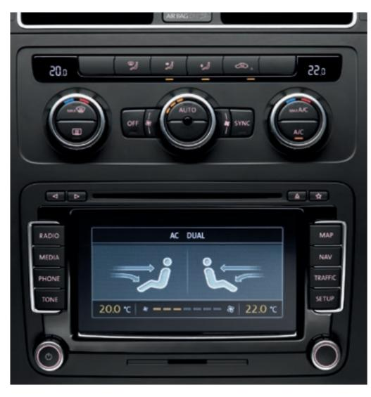
(S) Climate control – 2Zone electronic air conditioning controls the temperature electronically and divides the interior into two different climate zones, enabling the driver and front passenger to adjust the temperature, air supply and distribution to suit their individual preference. An air quality sensor continually monitors the outside air, automatically activating the interior air recirculation if necessary. Image shown features optional RNS 510 touch-screen DVD navigation/DAB radio system.
