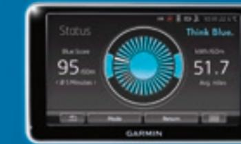
The 'Think Blue' Trainer helps you achieve an efficient driving style by analysing accelerating and braking characteristics, and providing valuable tips on how to adopt a more ecological and cost-saving driving style.
