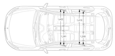
All measurements in millimetres. The dimensions shown are mean values and apply to standard-specification, unladen vehicles. Dimensions may vary slightly depending on the engine. Please consult your Retailer for further information
