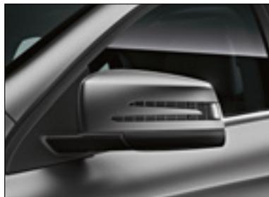
Automatically dimming driver's exterior mirror
