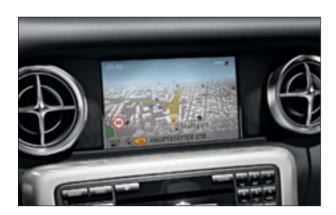
The information from Speed Limit Assist is shown both in the instrument cluster and on the COMAND Online central display
