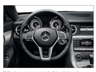
Multifunction sports steering wheel with a flattened bottom section.
