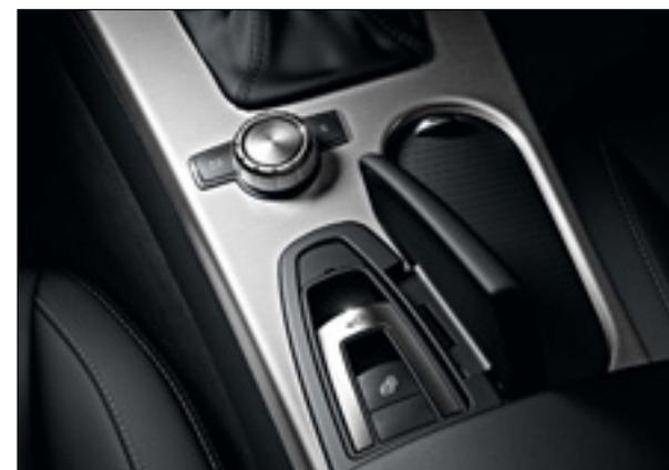
Roof control unit and Controller.
