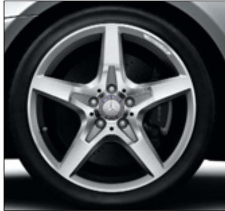
5-spoke AMG light-alloy wheels, high-shheen, with 225/40 R 18 front and 245/35 R 18 rear tyres (AMG Line, Code 782).
