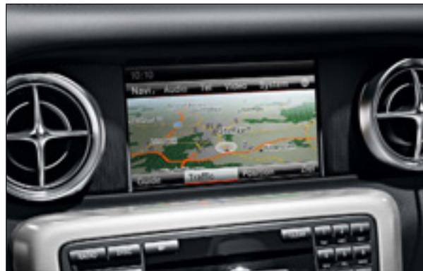
The optional COMAND Online system includes a high-resolution 17.8 cm display with TFT technology which provides a clear overview of all the system functions.
