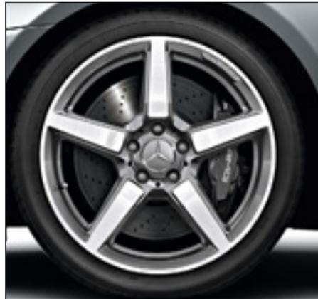
5-spoke AMG light-alloy wheels, painted titanium grey, high-shheen, 235/40 R 18 front and 255/35 R 18 rear tyres (standard for SLK 55 AMG, Code 790).
