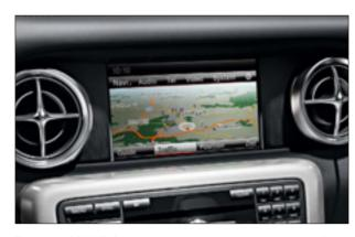
The optional COMAND Online system includes a high-resolution 17.8 cm display with TFT technology which provides a clear overview of all the system functions.
