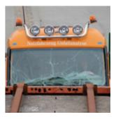
Bending and breaking: roof-mounted headlamp holder in a crash test.
