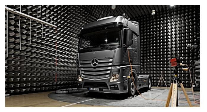
EMC testing in a hall specially shielded against external electromagnetic interference
