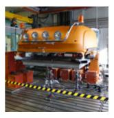
The hydropulse test stand simulates potholes and poor road conditions.
