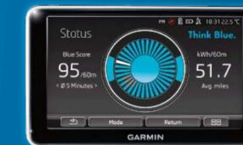
'Think Blue' analyses accelerating and braking characteristics, and provides valuable tips on how to adopt a more efficient driving style.
