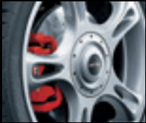
16-inch sport brake with perforated and grooved front brake discs
