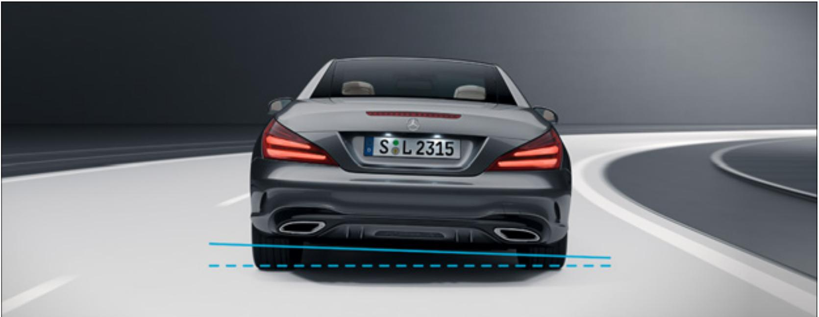
ABC is arguably the highest-quality suspension system on the market, offering the ultimate in driving dynamics and comfort by automatically adapting the suspension setting to the prevailing driving situation.
