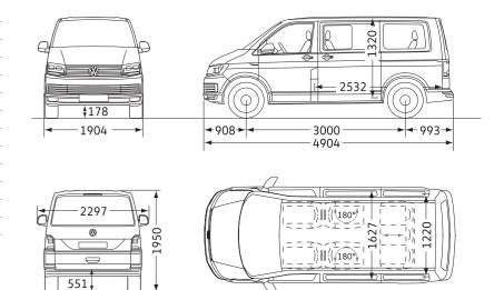
Please note: Vehicle drawings are not to scale. All dimensions are in millimeters (mm), unless otherwise stated. The height measurements listed may vary by  $\pm$  50mm depending on model and equipment fitted.
