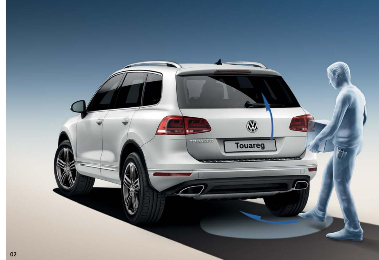
**02** The **hands free tailgate opening** function enables you to open the tailgate without having to make contact with your Touareg as long as you have the key in your possession. A small foot movement triggers sensors at the vehicle's rear and the rear tailgate will open out. Hands free tailgate opening is a function of the optional **keyless entry/keyless start and full electric tailgate operation**. Optional on SE and Escape models.
