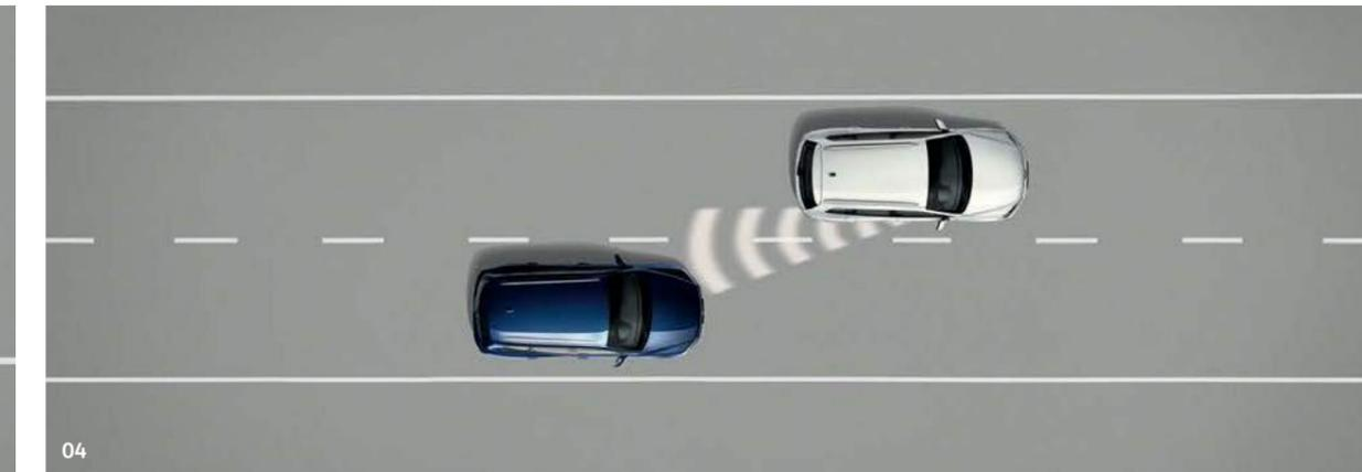
**03 Automatic Post-Collision Braking System** starts the brake operation after impact to help avoid further collisions. Supported by the airbag sensors, the system automatically initiates braking after the vehicle suffers a collision, and brakes for as long as necessary to reduce the speed of the vehicle to approximately 6mph in order to help prevent or help minimise the severity of subsequent collisions. Standard on all models.
