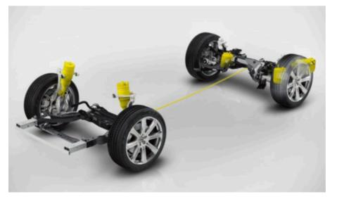
Choose the off road mode and the air suspension will raise the car by 40 millimetres. Hill Descent Control is activated at the same time: the car brakes for you on steep gradients – all you need to do is steer. The off road mode gets your XC90 to navigate challenging terrains – all you need to do is turn the elegant drive mode selector to the desired position. T6 AWD | Inscription | Crystal White | Exterior Styling Accessories Rugged | 22" 6-Double Spoke Matt Tech Black/ Diamond Cut
