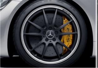
AMG high-performance ceramic composite braking system
