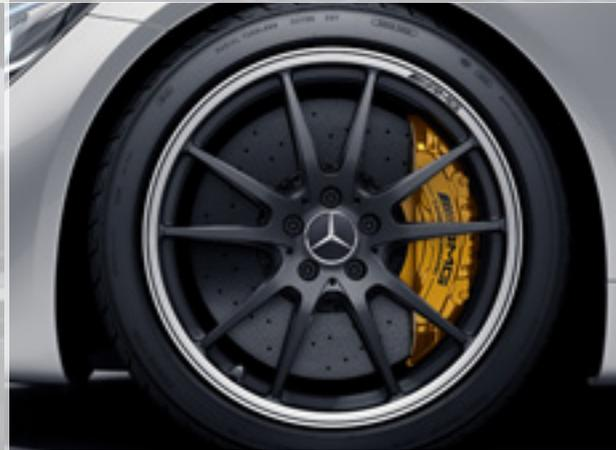
AMG high-performance ceramic composite braking system
