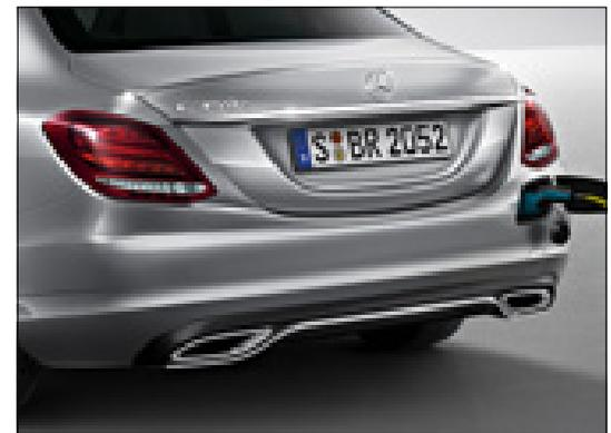
Visible twin-pipe exhaust trim integrated into rear bumper
