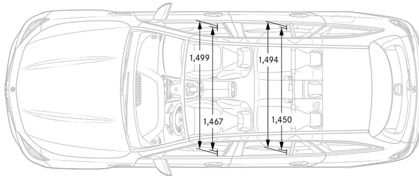
All measurements in millimetres. The dimensions are mean values and apply to standard-specification, unladen vehicles. Please note that wheels shown do not form part of standard UK specification. The figures on pages 95–102 are correct at time of publication. Please refer to the government website for latest data – <http://carfueldata.direct.gov.uk/>
