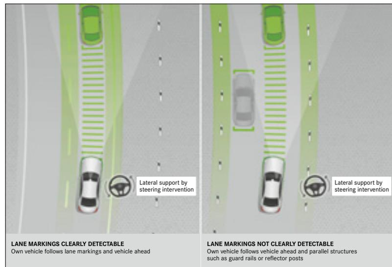
Active Distance Assist DISTRONIC – Active Steering Assist – Active Speed Limit Assist
