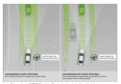
Active Distance Assist DISTRONIC - Active Steering Assist - Active Speed Limit Assist
