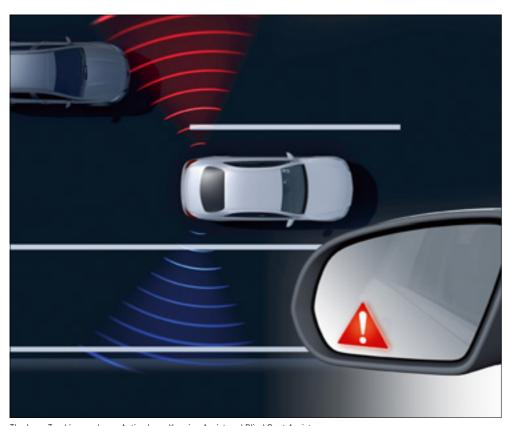
The Lane Tracking package: Active Lane Keeping Assist and Blind Spot Assist
