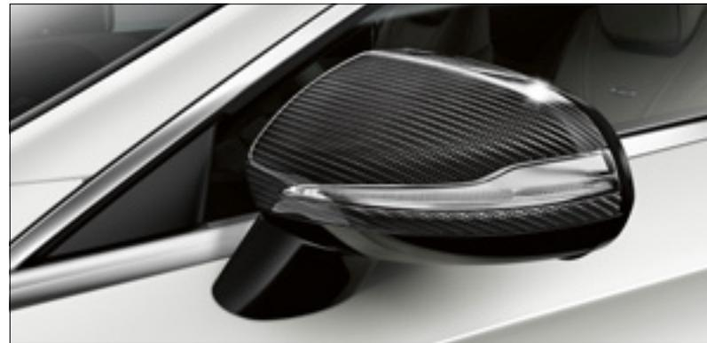
Exterior mirror housing in carbon fibre
