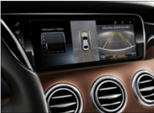
360° camera provides visual support when manoeuvring
