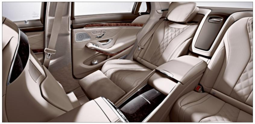
Reclining rear seat with additional leg and footrest (part of the Rear Seat Reclining package), as well as individual rear seats with folding rear tables (part of the Individual Rear Seats package) shown
