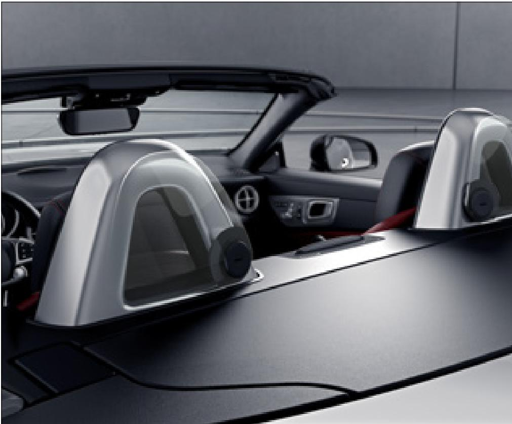
Defy the elements. To help you enjoy top-down motoring as often as possible, the SLC offers AIRGUIDE – a pair of transparent draught deflectors discreetly located behind the seat headrests. When required, these manually pivot into position helping to minimise turbulent air flow and noise within the cabin.
