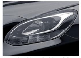
Halogen headlamps with integrated LED daytime running lamps
