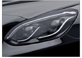
LED Intelligent Light System with Adaptive Highbeam Assist Plus
