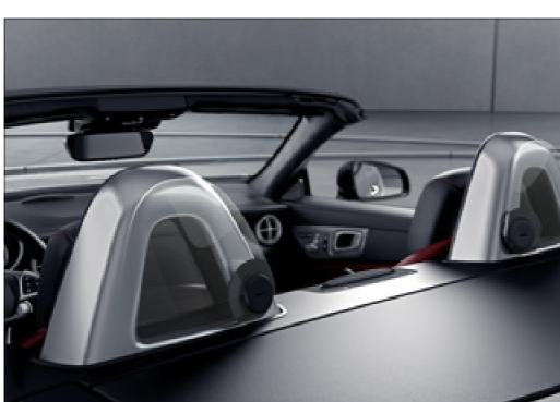
Defy the elements. To help you enjoy top-down motoring as often as possible, the SLC offers AIRGUIDE – a pair of transparent draught deflectors discreetly located behind the seat headrests. When required, these manually pivot into position helping to minimise turbulent air flow and noise within the cabin.
