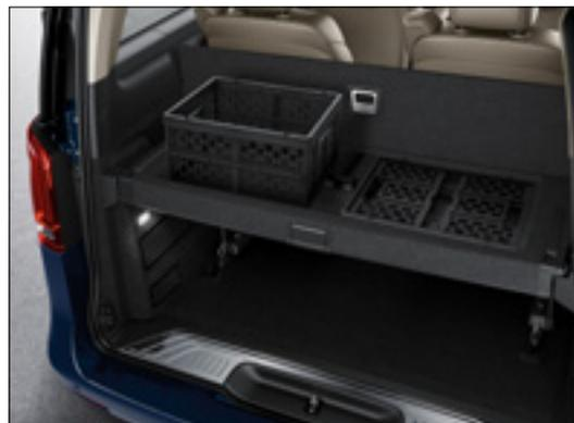
Load compartment divider with two folding boxes
