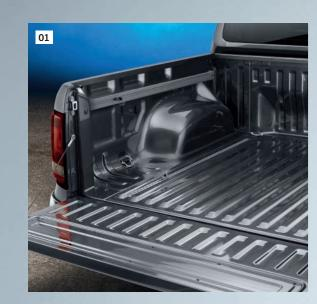
01 Wide and flat tailgate. The standard tailgate sits just 780mm from the ground. When folded flat, it's able to support weights of up to 200kg and serve as a load bed extension.
