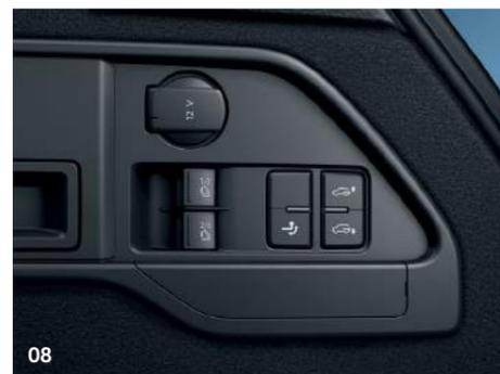
**08** The **control panel** in the boot automatically releases the rear seat backrest and the optional towbar if fitted, and also lowers the rear of the vehicle for easier loading and unloading.
