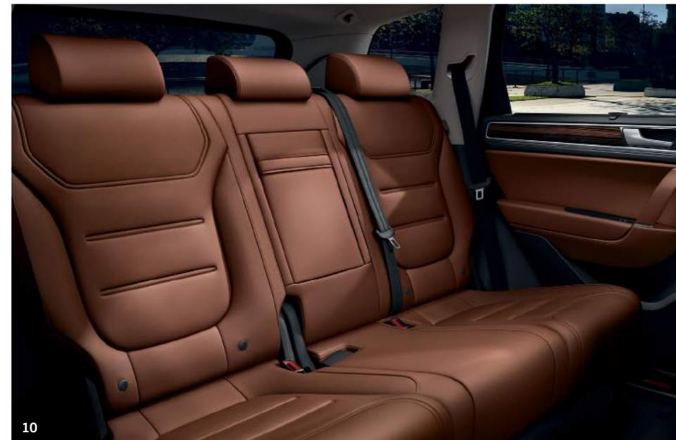
**10** The **modular design of the rear seating area** enables each rear seat to be moved lengthways and the backrest inclined to three different angles. When moved forward, this increases the boot volume from 580 to 679 litres.
