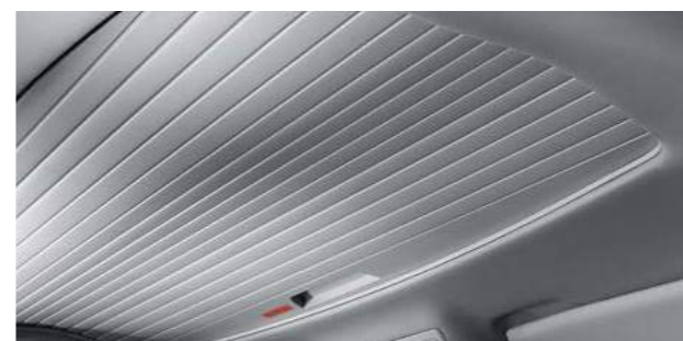
Sliding screen between cab and pop-up roof.
