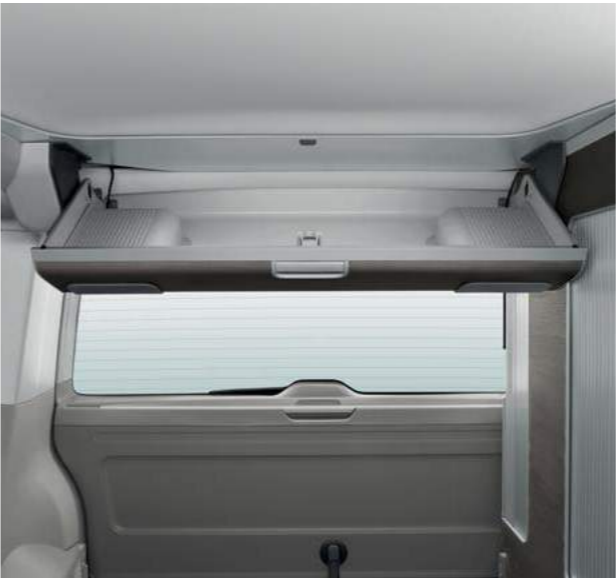
Drop-down rear compartment incorporating rear speakers.
