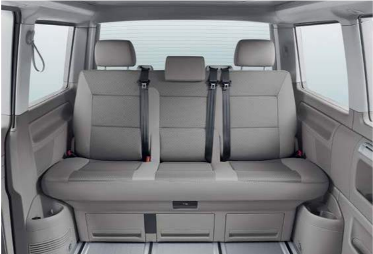
Optional folding three-seat rear bench with individual head restraints, seatbelts and under-seat storage.
