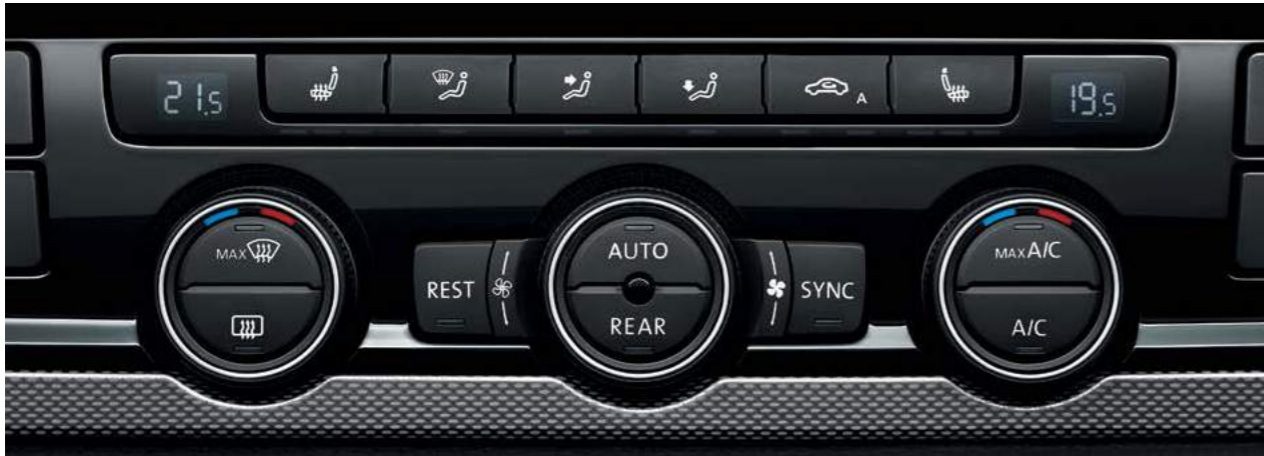
Climatronic three-zone automatic air conditioning and heated driver and front passenger seats.
