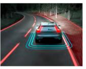
Run-off road Mitigation Stay safely on the road with this Volvo Cars safety innovation. If Run-off road Mitigation detects you're about to leave the road unintentionally, it uses steering input and, if necessary, brake support to guide you back on track.
