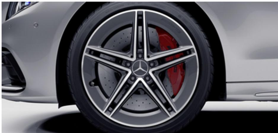
**RSW** 19"/20" AMG alloy wheels – 5-twin-spoke design, aerodynamically optimised, painted tantalite grey with a high-shine finish
