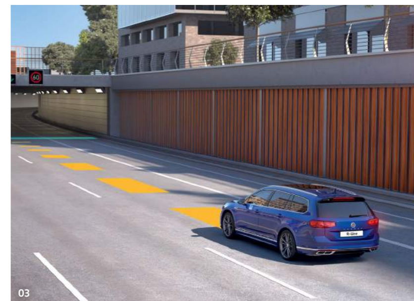
03 Adaptive Cruise Control (ACC) is a radar sensor controlled distance monitoring system that utilises a front mounted camera to set a distance to the vehicle in front and maintain it up to a predetermined set speed by automatically accelerating and braking as necessary. The system adds speed and cornering assistance by using information from the vehicle's navigation system if fitted. Standard on all models.
