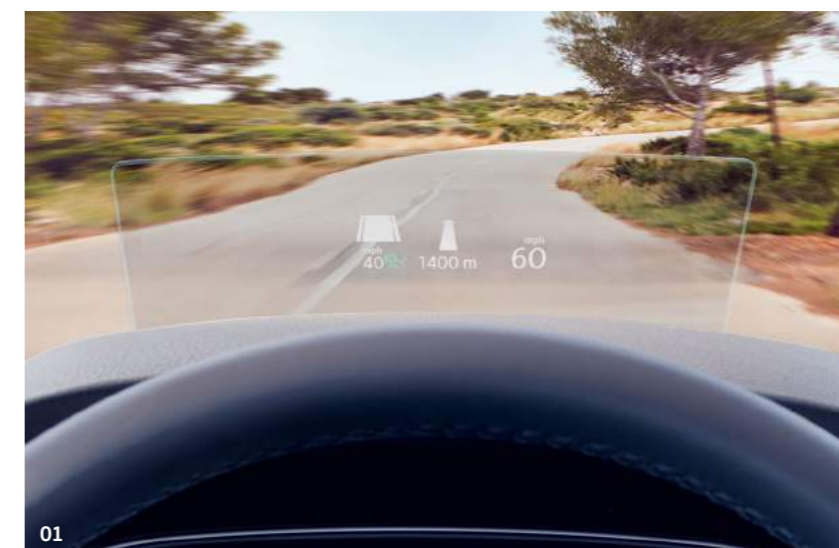
01 The optional Head-up Display 1 presents driving information directly in your field of vision. Speed, traffic signs and information about the assistance systems, as well as warnings and navigation data are projected on to the high-quality retractable screen transparently displayed in front of the windscreen, enabling you to read everything clearly while keeping your focus on the road ahead. Optional on SE, SEL, R-Line, GTE, GTE Advance and Alltrack models.
