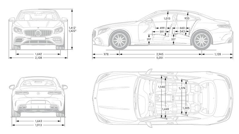
'Suspension mode 'Sport' <sup>2</sup>Suspension mode 'Comfort' All measurements in millimetres. The dimensions shown are mean values and apply to standard-specification, unladen vehicles. The figures on pages 45–47 are correct at time of publication. Please refer to the government website for latest data – http://carfueldata.direct.gov.uk/
