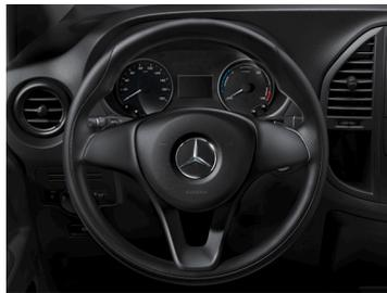
Height and rake adjustable steering wheel
