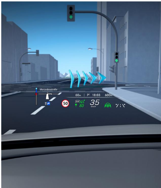
**MBUX augmented reality head-up display** makes the front windscreen part of the digital cockpit. With the help of transparent projections onto the windscreen, the driver's field of vision is enhanced with relevant information about the current driving situation.
