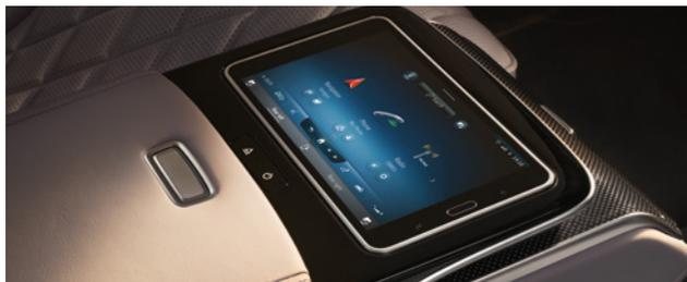
**MBUX 7-inch rear tablet** with the ability to control many on-board functions.
