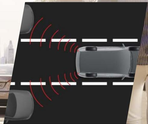
*The Blind Spot Monitor allows the driver to manoeuvre more safely during lane changes. If the rear-mounted radar sensors detect a vehicle in your side or rear blind spot, a warning indicator will illuminate on the appropriate side mirror. Should you indicate to change lanes and a vehicle is in your blind spot, the warning indicators will flash to alert you that a lane change should be avoided.*
