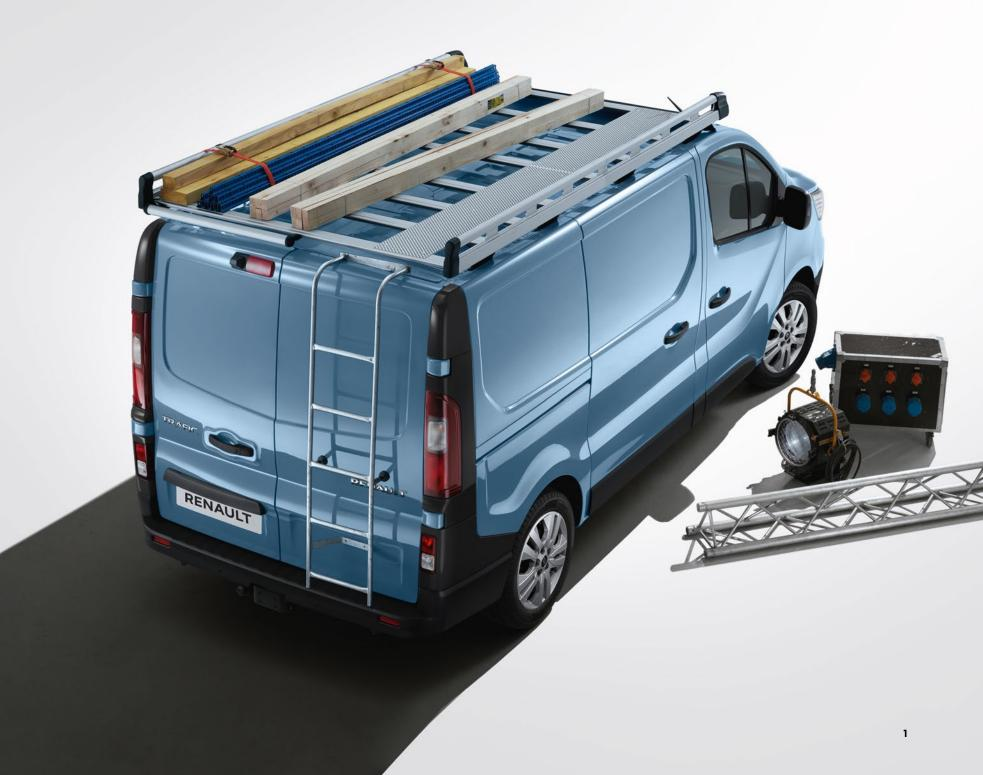
1. aluminium roof rack - roof rack track galvanised ladder
