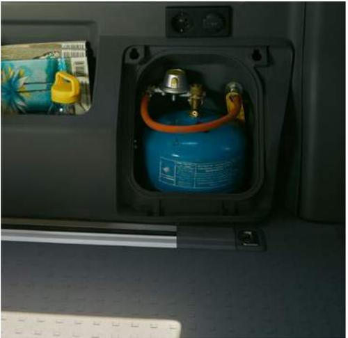
**Gas storage compartment.** Under the hermetically sealed cover, an optional 1.8 kg Campingaz gas cylinder<sup>1</sup> can be securely attached to straps and connected to the gas hose.
