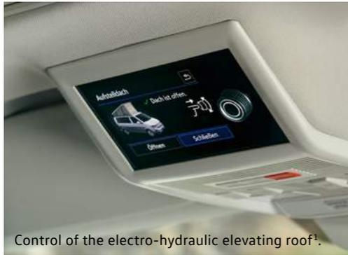
Control of the electro-hydraulic elevating roof<sup>1</sup>.
