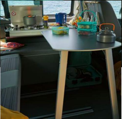
**Mini-kitchen with hinged folding table.** Stowed safely in the sliding door during the journey, the versatile folding table can be hooked into the guide rail of the folded-out mini-kitchen and placed on two legs if required.
