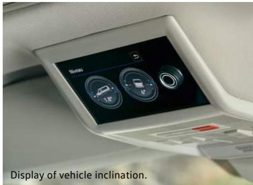
Display of vehicle inclination.
