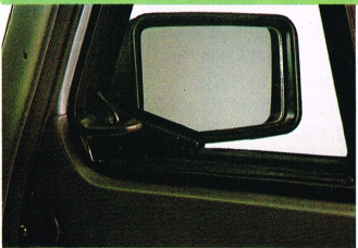
A feature normally associated with bigger cars: a driver's door mirror you adjust from the inside.
