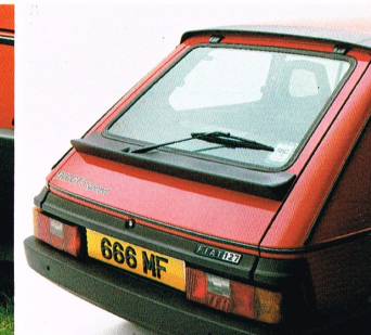
A hatchback with a difference: a rear wash/wipe to increase visibility and two rear spoilers to decrease wind resistance.
