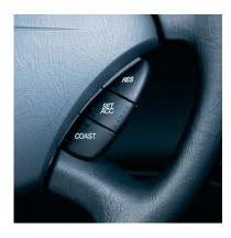
> Cruise Control. This fully integrated cruise control system features steering wheel mounted controls for driver convenience.
