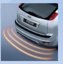
> Reverse sensing system. This system features warning tones to assist the driver when reversing and parking in tight spaces.
