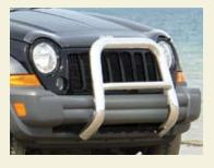
**Nudge Bar\*** adds extra style to your Cherokee's front end. This highly polished guard features a unique one-piece design that ensures a uniform fit.
