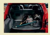
Moulded Cargo Tray<sup>+#</sup> fits in the rear cargo area to help protect carpeting. Skid-resistant, thermoplastic tray is available in matching interior colours. Features the Jeep logo and an embossed area to access the floor tie-downs.
