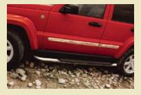
Chrome Tubular Side Steps complement the Nudge Bar and provide easier entry and exit to your Cherokee. Extra-wide stepping surfaces help prevent slipping. Available in Silver, Chrome and Grey steel or Silver aluminium.
