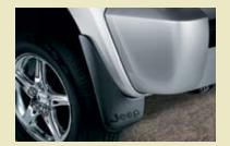
Deluxe Moulded Splash Guards provide excellent protection for the rear fascia. Made of a composite of TPO plastic and TPR rubber to be strong, yet flexible. Available in front and rear pairs in Black, Medium Grey and Dark Slate to match body cladding. Rear splash guards feature the Jeep logo. Not available for Renegade.
