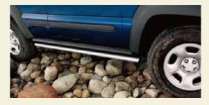
**Rock Rails** are production style and are constructed of heavy-gauge steel. They also provide added lower bodyside panel protection when off-roading. Available in Silver.
