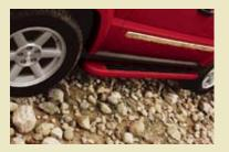
Moulded Running Boards can take the pounding you dish out. Skid-resistant surfaces help ensure easier entry and exit, especially in slush and snow. Moulded Running Boards include front mud flaps. Available primed to match body colours, Black or Grey to match Sport body cladding.
