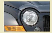
Headlight Protectors help to protect your headlamps from damage and dirt caused by loose gravel and bugs. Made of tough, shatterresistant acrylic these protectors provide excellent durability in both on and off road conditions.
