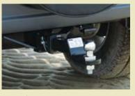
Tow Bar<sup>\*</sup> comes as a complete towing solution. Tow Bar is rated to a maximum towing capacity of 2,800kg. Kit includes tow bar, tongue, tow ball and wiring harness.
