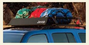
**Roof Top Cargo Basket**<sup>#</sup> has high sides to help secure cargo and features a front air deflector with Jeep logo. Mounts to standard equipment side rails or Sport Utility Bars (sold separately).
