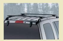
Sport-Utility Bars are built of heavy-duty Silver anodised aluminium. T-slots allow for quick carrier installation. Bars attach to the **Production Roof Rack Side Rails** and accommodate all Jeep Carrier Accessories. Set of two.
