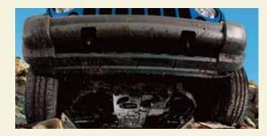
Skid Plates for the front suspension, transfer case, engine and fuel tank offer heavy-duty protection for these underbody components when covering rough terrain.
