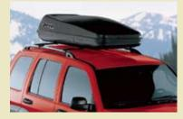
Roof Box Cargo Carrier attaches to either Production Roof Rack Cross Rails (shown) or Sport-Utility Bars. Tough, locking thermoplastic carrier keeps cargo dry and secure no matter what the weather. Features quarter-turn installation, gas-cylinder opening system and Jeep logo. Available in two sizes.
