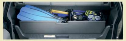
**Cargo Organiser**<sup>†#</sup> makes the most of your Cherokee's cargo area. The organiser's interior space can be reconfigured by raising and lowering its dividers — it can be used as a divided storage bin forming up to three compartments with additional storage underneath, or folded flat and used as a security cover.
