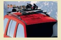
Roof-Mount Ski and Snowboard Carriers" help you get to the slopes in style. Carrier holds up to six pairs of skis or four snowboards, or a combination of the two. Feature Silver anodised aluminium construction and corrosion-resistant lock covers.
