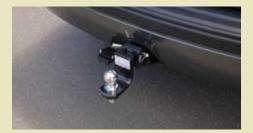
Tow Bar<sup>‡</sup> comes as a complete towing solution. Tow Bar is rated to a maximum towing capacity of 3,500 kgs. Kit includes tow bar, tongue, tow ball and wiring harness.
