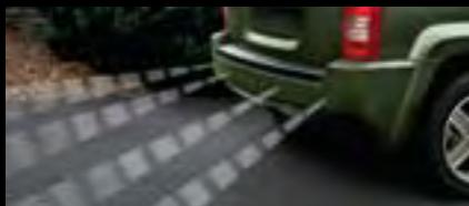
REAR PARK ASSIST SYSTEM.<sup>(1)</sup> Advanced system uses sound waves and audio-visual indicators to manoeuvre in tight spaces at parking speeds.
