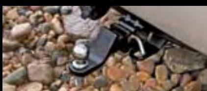
TOW BAR KIT.<sup>(2)</sup> This towing kit includes tow bar, tongue, tow ball and wiring harness.
