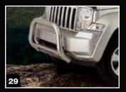
29. CHROME NUDGE BAR. This heavy-duty stainless steel nudge bar helps protect the front end of your vehicle from minor bumps and scratches.
