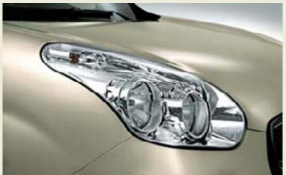
The characteristic, three-dimensional, wrap-around headlights stretch back at the top to incorporate the indicators.
