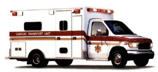
Econoline E-450 Super Duty RV Cutaway with 7.3L Power Stroke turbo diesel and Ambulance Prep Package (aftermarket equipment shown). Econoline is a mainstay for the health care industry.
