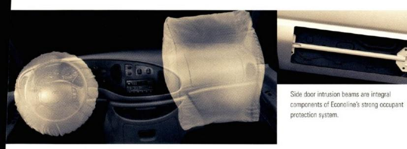
Second Generation Depowered airbags are designed to further enhance protection for driver and passenger while also reducing the risk from potential airbag inflation injury.
