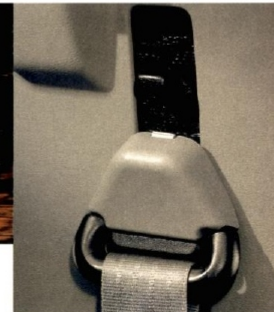
Shoulder belts have D-ring height adjusters to satisfy the comfort needs of short and tall people alike.
